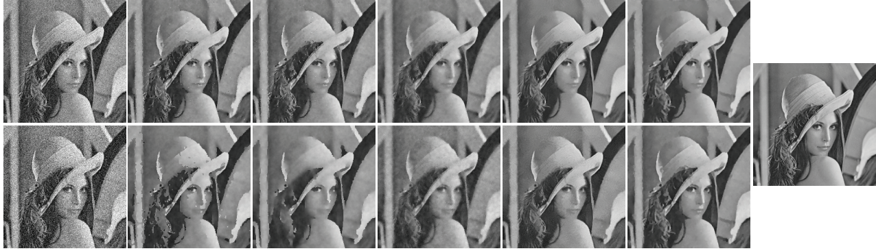
Fig. 2. Results of the five algorithms on the “Lena” image with the noise \sigma = 20 (the first row), and \sigma = 30 (the second row). From left to right: the noisy images, the results by GC, BP, BF, NL, and our algorithm, and the original noise-free image
